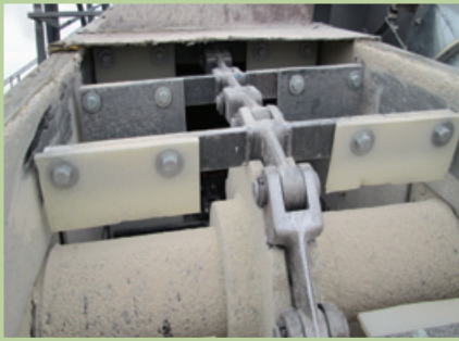
4B142HA Chain With UHMW Paddles On Flat Bar Flights Moving 20K BPH Of Corn
