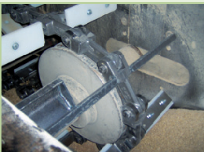
4B142HA Chain With Return Cup And UHMW Paddles On Flat Bar Flights - Tail End Shown
