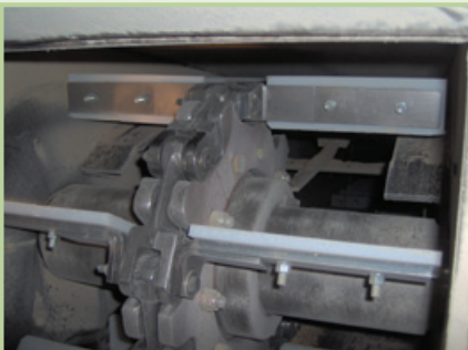
4B142HA Chain With UHMW Paddles On Flat Bar Flights - Drive End Shown
