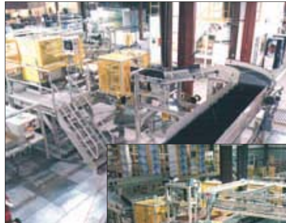
PALLETIZER Fully automated bag palletizer
