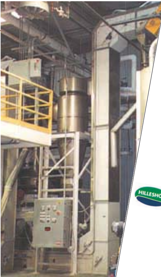
Vertical Sidewall Belt Conveyor – Kemin Industries, Des Moines, IA
