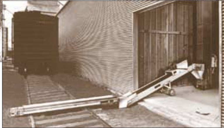
Early car unloader and booster conveyor.
