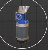
Micro ingredients are weighed in the stainless steel drum, which rotates to discharge into a transfer conveyor.
