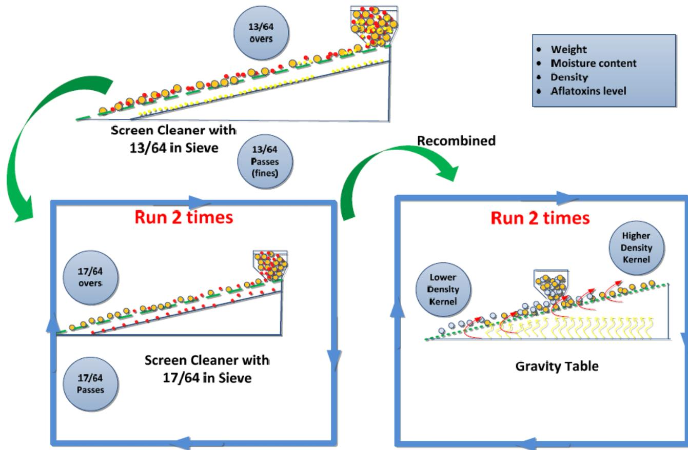
Figure 3. Diagram showing size and density segregation tests conducted at a commercial inbred seed processing facility.
