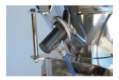
NTP 18 mounted on a hopper using the Stick and Shake system.
