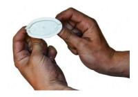
Adhesive strips are first applied on the perimeter of the mounting base.
