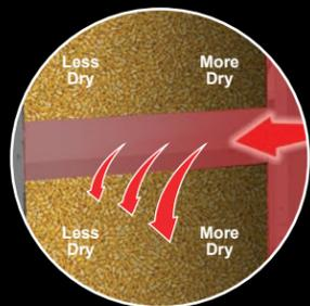
Competitor duct designs are straight, which may fail to dry uniformly across the grain column.
