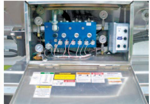
Junction boxes include wiring diagram labels inside. All utility boxes are manufactured from aluminium and all boxes are positioned for easy access.
