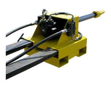
The Fork Devil Forklift Mounted Hopper Gate Opener is one of the most economical openers we manufacture, but it's just as powerful as the rest. This unit's hydraulic motor is powered by the hydraulic system of the forklift or other fork equipped device via the auxiliary hydraulic ports. This makes the Fork Devil a great solution where power options such as air and electric are not available.
