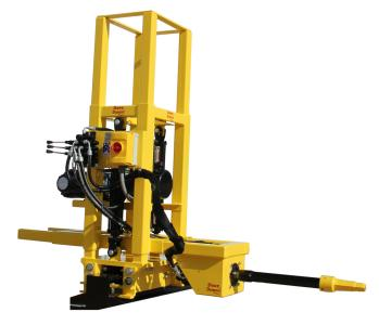
The Multi-Position Beam Mounted Hopper Gate Opener is the optimal tool for opening the toughest hopper gates in a busy railyard. The unit features an electric over hydraulic system with powered height adjustment as well as forward and retract motion. This enables simple lever-operated adjustment to fit a wide range of railcar capstan heights and depths. The free-moving trolley system rolls easily and allows for moving trains and capstans.
