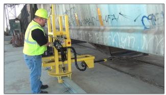
The unit is easily modified to fit into most unloading areas with customized shaft lengths. In addition, a rotation option is available to completely remove the drive shaft from the walkway. This is especially helpful in tight layouts, as this option also prevents the driveshaft from making contact with the railcar.
