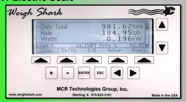
The kW Scale allows you to measure weight for your augers and conveyors by measuring the amp draw.
