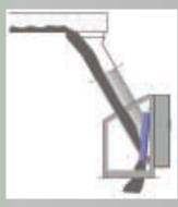
**Weigh Shark** SI Dry Solids Impact Flow meters are designed for operation in conjunction with Dry, Solid material flowing by Gravity. It is designed for operation under normal atmospheric pressure and should <u>never</u> be operated in conjunction with positive AIR pressure or vacuum systems. This is precise measurement device incorporates strain gauge load cells to measure force of impact against a metal plate must be free of external factors.
