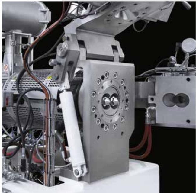
Detail of the extruder head showing the two extrusion screws characteristic of the TT92.
