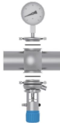
*The process connections offer the option of holding up to two components in one VARINLINE® housing*
