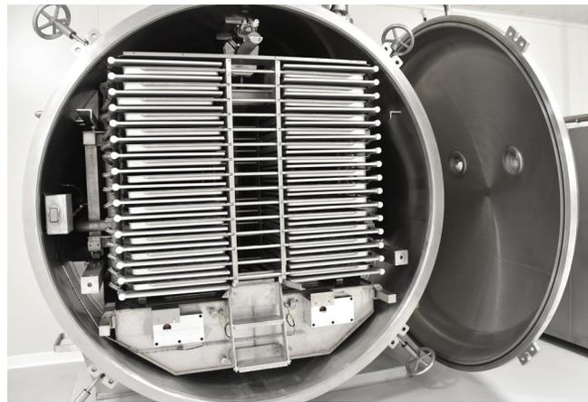
The overhead rail system for loading and unloading, and the Continuous De-Icing system, enable a changeover time between batches of under 30 minutes.
