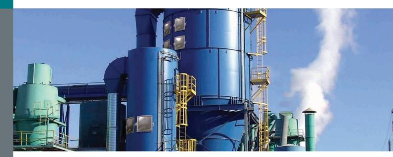
As the cost of energy continues to increase, plant managers are continually looking for ways to reduce power consumption. Within the Schenck Process filter portfolio is the unique MCF PowerSaver®, a dust collector that can save up to 50% of operational costs by using medium pressure air at only 7 PSI for the cleaning cycle. The air is provided by its own blower, therefore no plant compressed air is used, potentially freeing up the expense to produce air for other applications.
