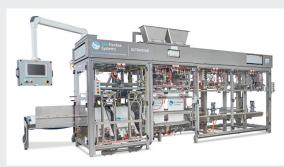
UltraStar with its quad MasterWeigh 60-series scales can run up to 38 bags/min.
