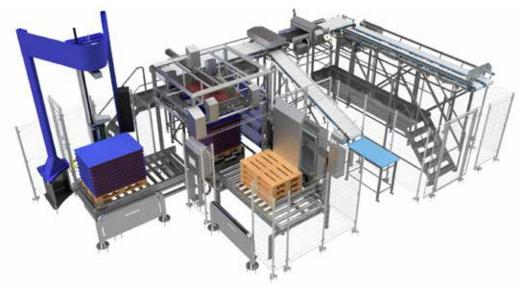
The stacking unit picks the blocks up fror the table one by one and automatically stack them on a pallet. The system stacks the block in a criss-cross layout creating a more stabl pallet, which is safe to store and transport.
