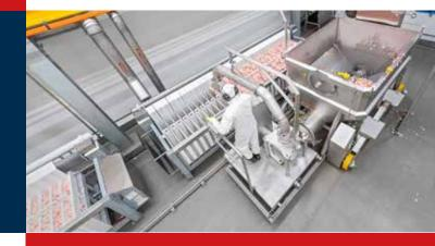
When loading a plate freezer, it is important to choose the correct filling system that suits the raw material requirements.
