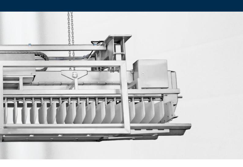
We offer equipment and systems for automating the plate freezing process from unloading the freezers to palletizing, weighing and wrapping the frozen plates.
