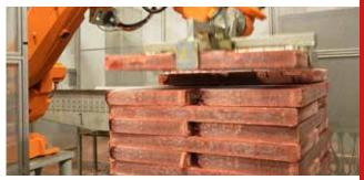
Stacking with robot, automatic manipulator or manual stacking
