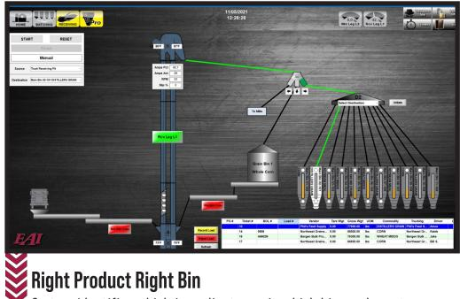
System identifies which ingredients are in which bins and creates a pop up notification if the user tries to put a different ingredient into that bin. This feature will help prevent the operator from putting an ingredient in the wrong ingredient bin.
