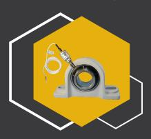
The HB21 sensor screws into an existing bearing's grease fitting and is ideal for bearings, gearboxes, bucket elevators, mills, grinders, conveyors, mechanical drives, and most other handling equipment. Discover the versatility of HB21 bearing temperature sensors, available in Type-T, RTD, PTC, and DigiMax versions.
